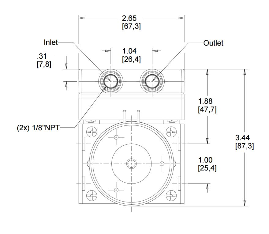
\* Dimensions are in inches [mm]. DV1032200 or DC1032200 shown. 5.57 [141,5] dimension is motor selection dependent.
